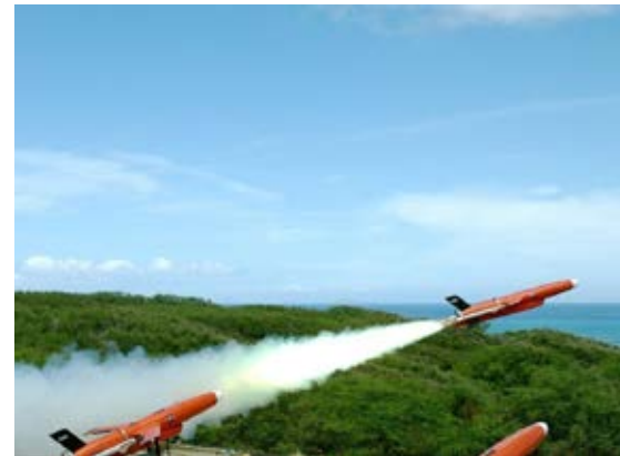
Drone launch with JATOs -Photo courtesy of Pacific Missile Range Facility, Barking Sands, Hawaii
